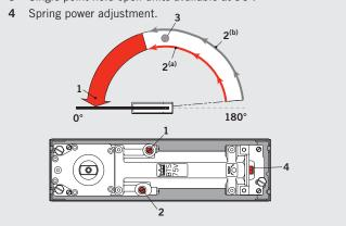
**NOTE:** If door hardware or adjacent structures interfere with maximum opening, an auxiliary stop is required.
