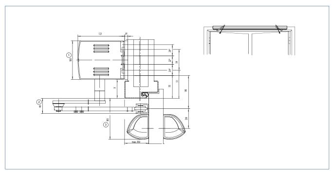
X = Spindle extension | \* = Installation with mounting plate | 1 = Space needed for TSA 160 NT | 2 = Space needed for link arm | 3 = Space needed for sensor strips
