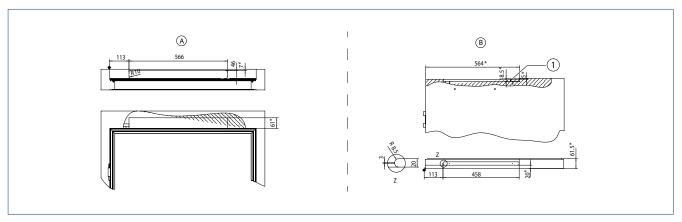
A = Cut-out for drive | B = Door cut-out | 1 = Cut-out for lever | \* = Dimensions or positions may deviate depending on the door type.
