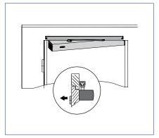
Door leaf installation with guide rail / roller guide
