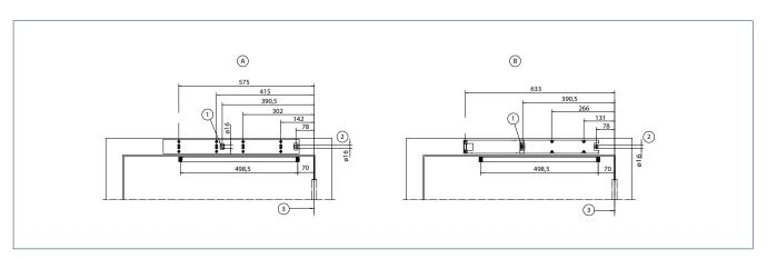
A = Installation with mounting plate | B = Direct installation | 1 = Concealed line-feed for low-voltage connection | 2 = Concealed line-feed for low-voltage connection and mains cable | 3 = Dimensional reference centre of hinge
