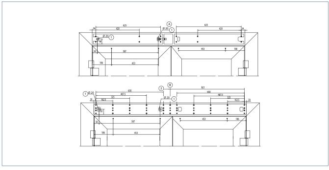
A = Direct installation | B = Installation with mounting plate | 1 = Concealed line-feed | 2 = only needed for B>2000
