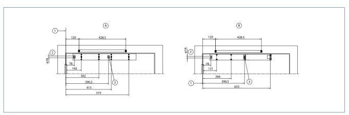
A = Installation with mounting plate | B = Direct installation | 1 = Dimensional reference centre of hinge | 2 = Concealed line-feed for low-voltage connection and mains cable | 3 = Concealed line-feed for low-voltage connection
