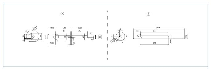
A = Frame cut-out  $\mid$  B = Door cut-out  $\mid$  \* = Dimensions or positions can deviate depending on the door type.
