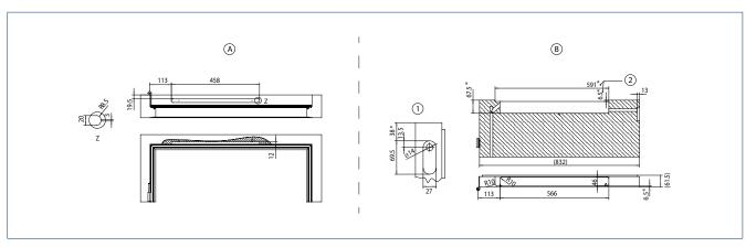
A = Frame cut-out | B = Door cut-out | 1 = Cut-out for programme switch (optional) | 2 = Cut-out for lever | \* = Dimensions or positions may deviate depending on the door type.
