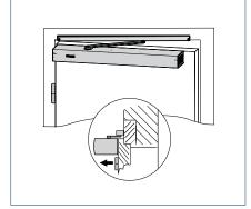
Door leaf installation with guide rail / roller guide
