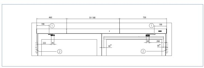
B = Hinge clearance | \*\* = Recommended size for installation of the GC 335 and GC 338 sensor strip | 1 = Hinge clearance | 2 = Dimensional reference centre of
