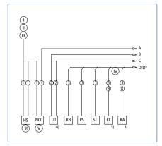
I = Power supply circuit 230 V / 50 Hz | II = Safety fuse 10 A | III = Connection value 300 W, 1.3 A for single, double leaf with manual passive leaf connection value 600 W, 2.6 A for double leaf | IV = And / Or | V = Option
