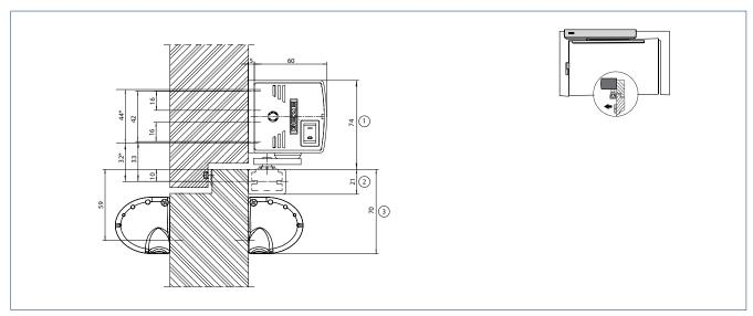
\* = Direct installation | 1 = Space needed for ECturn | 2 = Space needed for guide rail | 3 = Space needed for sensor strip
