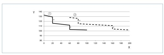
\* = Preload | X = Reveal depth (mm) | Y = Max. door opening angle (°) | 1 = Lever 330 mm | 2 = Lever 450 mm
