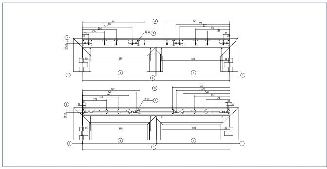
A = Installation with mounting plate | B = Direct installation | 1 = Dimensional reference centre of hinge | 2 = Concealed line-feed for sensors, electric strike, programme switch and lock switch contact | 3 = Concealed line-feed 230 V / 50 Hz | 4 = Door leaf width | 5 = Hinge clearance
