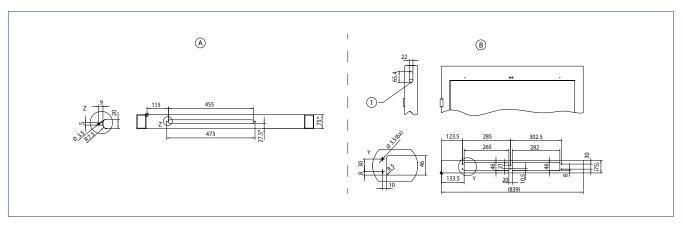
A = Door leaf cut-out | B = Door leaf cut-out | 1 = Cut-out for programme switch (optional) | \* = Dimensions or positions may deviate depending on the door type.
