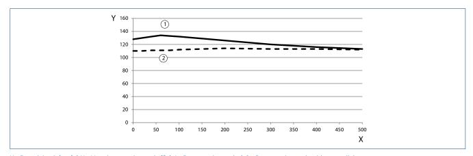
X = Reveal depth (mm) | Y = Max. door opening angle (°) | 1 = Door opening angle | 2 = Door opening angle with sensor link arm
