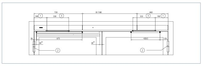
B = Hinge clearance | \*\* = Recommended size for installation of the GC 335 and GC 338 sensor strip | 1 = Hinge clearance | 2 = Dimensional reference centre of hinge | 3 = Lever length
