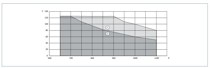
X = Door width (mm) | Y = Door weight (kg) | 1 = Area of application in low-energy mode | 2 = Area of application in automatic mode
