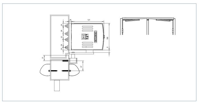
$<sup>^{*}</sup>$  = Installation with mounting plate and GC 338
