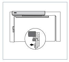
Transom installation with guide rail / roller guide
