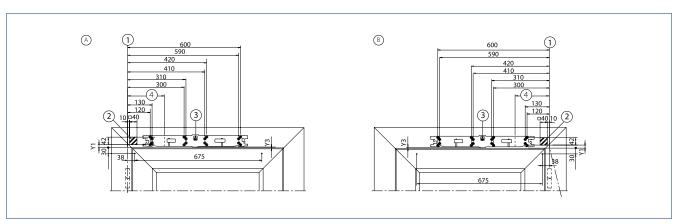
A = DIN left | B = DIN right | 1 = Dimensional reference centre of hinge / door frame bottom edge | 2 = Concealed line-feed possible in the hatched area, e.g. Ø 20 mm for network connection or low-voltage connection | 3 = Orientation arrow for clear positioning of the mounting plate | 4 = Hinge clearance
