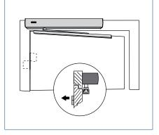
Transom installation with guide rail / roller guide
