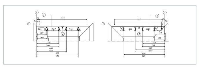
A = DIN left | B = DIN right | 1 = Dimensional reference centre of hinge / top edge of door | 2 = Orientation arrow for clear positioning of the mounting plate | 3 = Hinge clearance
