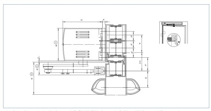
\* = Installation with mounting plate | 1 = Space needed for TSA 160 NT | 2 = Space needed for link arm | 3 = Space needed for sensor strips
