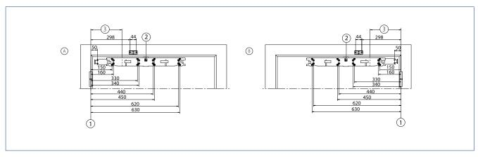
A = DIN left | B = DIN right | 1 = Dimensional reference centre of hinge | 2 = Orientation arrow for clear positioning of the mounting plate | 3 = Hinge clearance
