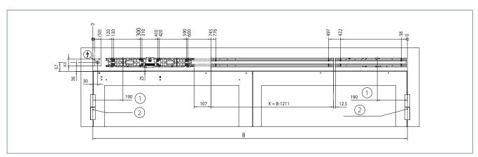
K = Position of the intermediate base plate | B = Hinge clearance | 1 = Hinge clearance | 2 = Dimensional reference centre of hinge
