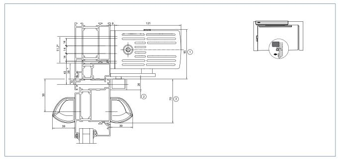
\* = Direct installation | 1 = Space needed for EMD-F/EMD Invers | 2 = Space needed for roller guide rail | 3 = Space needed for sensor strips
