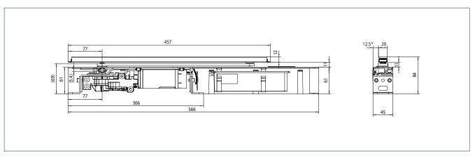
ECturn Inside Representation of a wooden door leaf, mirror-inverted for door frames
