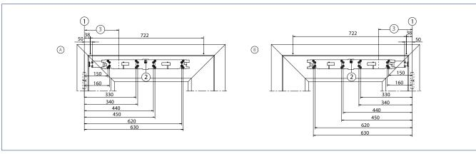
A = DIN left | B = DIN right | 1 = Dimensional reference centre of hinge / door frame bottom edge | 2 = Orientation arrow for clear positioning of the mounting plate | 3 = Hinge clearance
