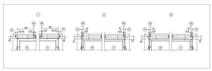
AV = Drive displacement | I = TSA 160 NT installation hinge side | II = TSA 160 NT installation opposite hinge side | III = TSA 160 NT-Z installation hinge side | I IV = Drive left - pulling I V = Drive right - pulling I VI = from top of leaf, dimension for spindle extensions must be added I VII = Cable exit
