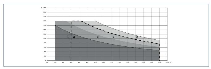
X = Door width (mm) | Y = Door weight (kg) | 1 = Dashed line: Area of application for installation with roller guide rail
