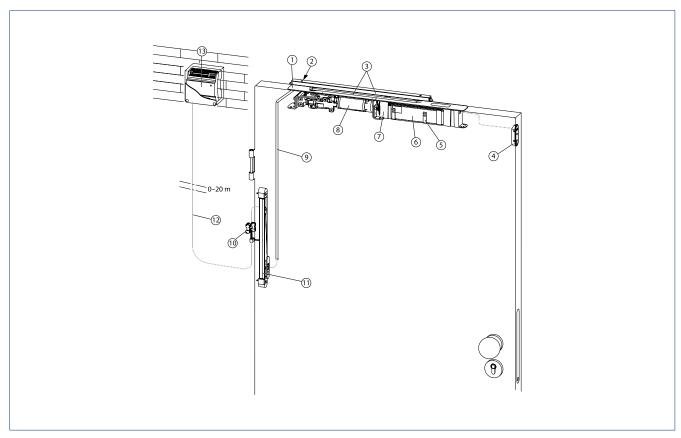
1 = Cover for motor gear unit | 2 = Back check | 3 = Guide rail and lever | 4 = Separate programme switch (optional) | 5 = Holder for rechargeable battery (optional) | 7 = Control unit | 8 = Motor gear unit | 9 = Power supply cable, inside door 2.5 m | 10 = Electric installation material | 11 = Drip loop (optional) | 12 = Power supply cable (on site) | 13 = Power supply (flush-mounted installation)
