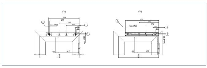
A = Installation with mounting plate | B = Direct installation | 1 = Dimensional reference centre of hinge | 2 = Concealed line-feed for sensors, electric strike, programme switch and lock switch contact | 3 = Concealed line-feed 230 V / 50 Hz | 4 = Door leaf width
