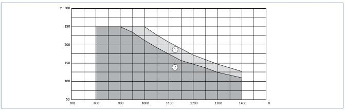
$X = Door width (mm) \mid Y = Door weight (kg) \mid 1 = Link arm \mid 2 = Roller guide rail$
