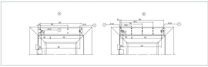
A = Direct installation | B = Installation with mounting plate | 1 = Concealed line-feed
